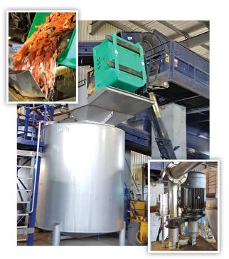
Salmon waste (top, right) is fed into an ensiling tank (center) equipped with an 18.5 kW stainless steel long shaft chopper pump (bottom, right). The "smooth purée" is then discharged into the pasteurizer.
